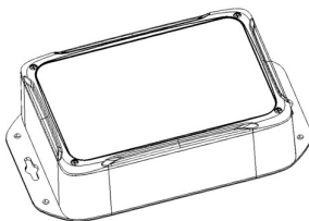
1X electrical box with drivers inside
